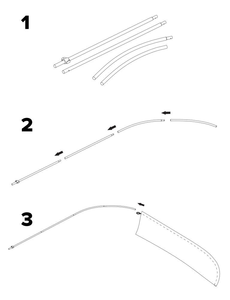
Make sure the pole is inserted to the end of the tunnel.
