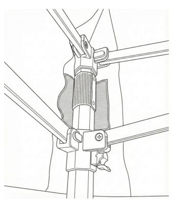
Tension the center pole by turning the crank handle.
